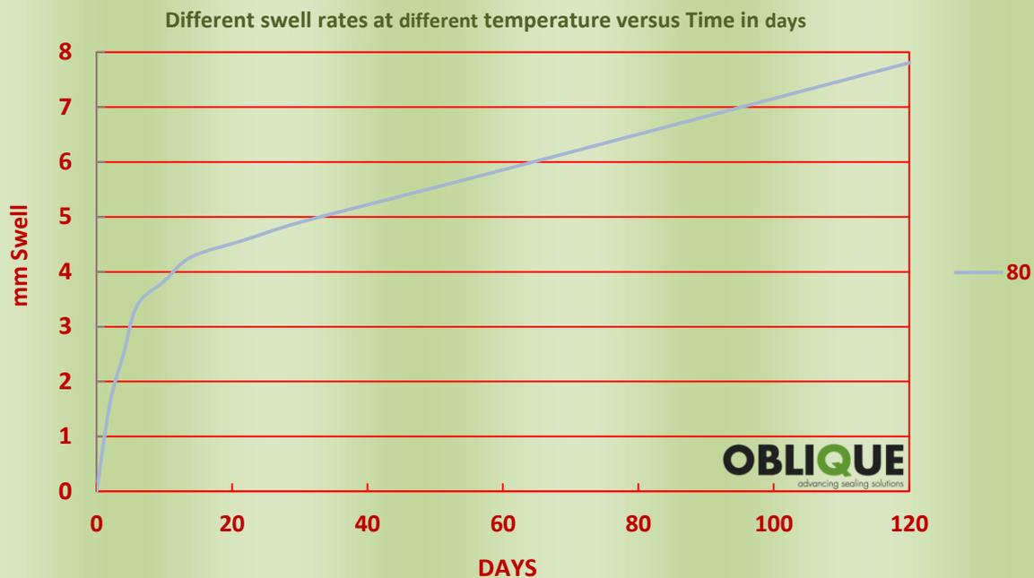
Fig 1 Standard water swelling elastomer Swell Curve
